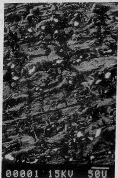
Fig. 8b SEM Micrograph Non- metallic inclusions distributed in ferritic and slag matrix
