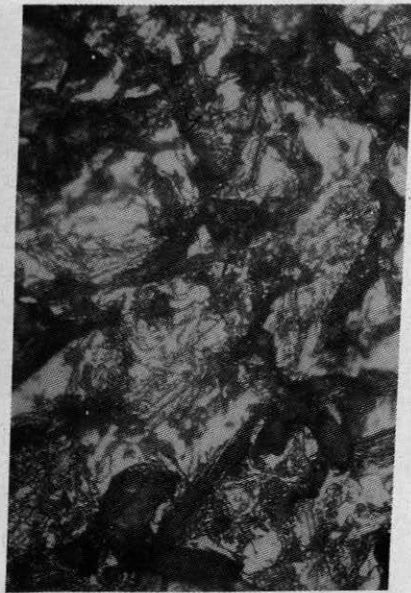
Fig. 2 Micrograph showing ferrite and coarse pearlite and coarse pearlite with slag. pockets 300X
